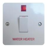
As part of the installation, there is a new hot water switch fitted in place of your old timer. **This should be left in the ON position at all times** and only be used to switch off your hot water completely for example, if you are going away for a few days and do not need any hot water. When the hot water is charging, the red light on the Water Heater Switch will be ON.
